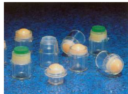
Developing the mounting system – the green modules were the prototype disposable collets (see also below)
